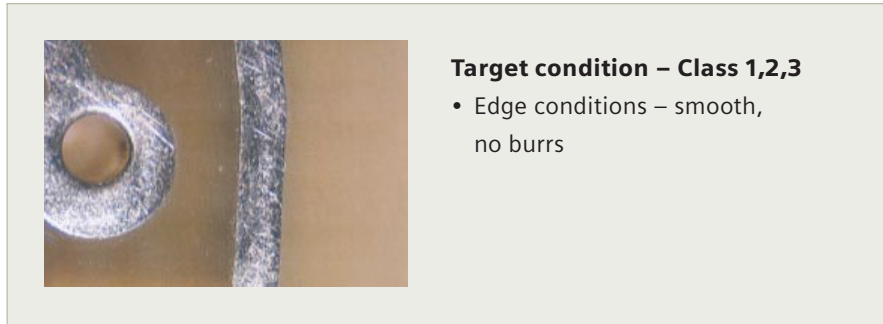
Figure 4. An example of an acceptable target condition, with a smooth surface appearance IPC-A-600K Section 2.1.2 Nicks . (Copyright IPC-A-600 reprinted with permission)
