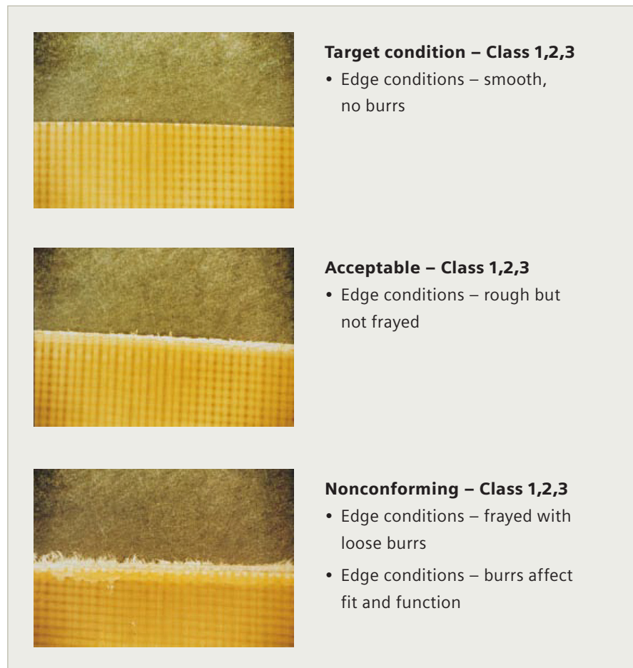
Figure 3. Nonmetallic burrs are representative of the quality of the depanelization process ( IPC-A-600K Section 2.1.1.1 Nonmetallic Burs ). These images are used as an example of acceptable final appearance and separate the quality into groups showing what is acceptable and what is nonconforming based on class 1, 2 or 3. This quality depends on the upkeep of the machinery used by the fab house. (Copyright IPC-A-600 reprinted with permission)
